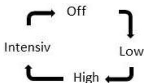
3. The third speed is timed, so the cooker hood will automatically revert to the second speed after seven minutes.
