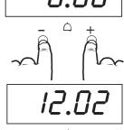
Immediately set the desired time with the "+" and "-" keys. The clock starts immediately.
