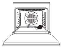
Carefully lever out the glass cover with a screwdriver.
