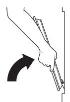
Gently lift the door and pull the hinges forward away from the door opening.
