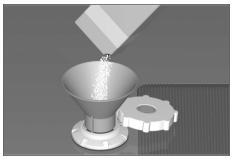
The LOW SALT indicator <u>B</u> on the front panel will light up initially but will extinguish again after a short period when the salt solution has become sufficiently concentrated.
